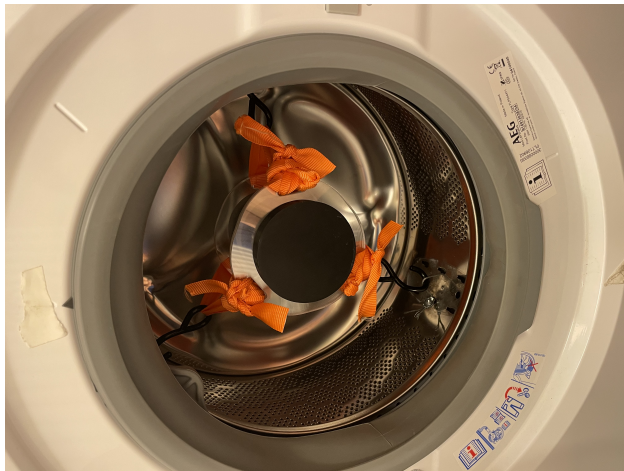
Figure 6.2: Front view of the centered weight setup in the washing machine
