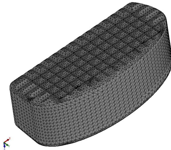
Figure 5.4: Mesh for the full design, using equilateral triangle element of 0.6mm side length with a 0.03mm tolerance, and the automatic transition.
