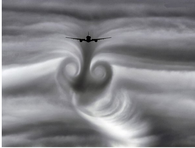
Figure 1.13: Visualization of the wake turbulence of an airplane ©Steve Morris
