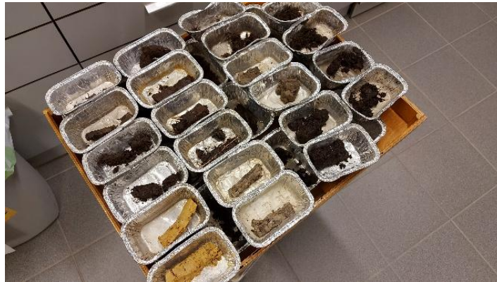
Figure A.4: Samples before heating process
