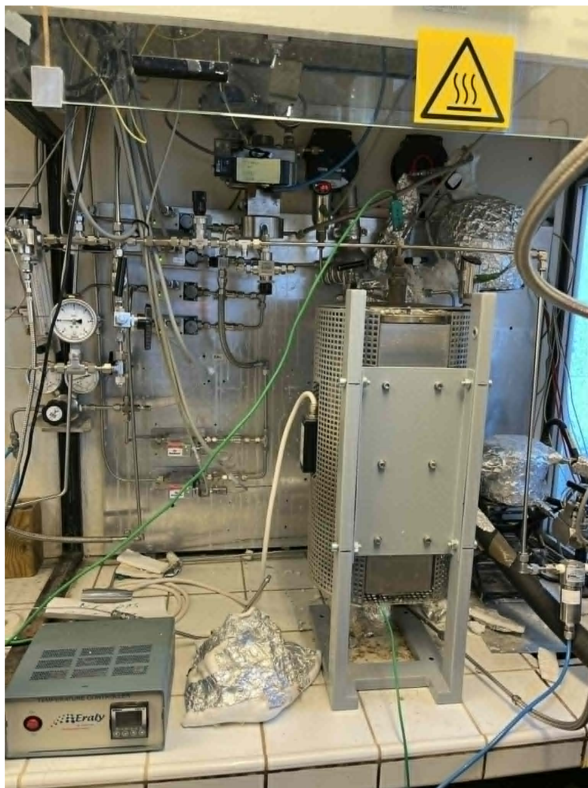
Figure 2.1: Picture view of the micro-fixed bed reactor set-up used to study the methanation of \text{CO}_2 .
