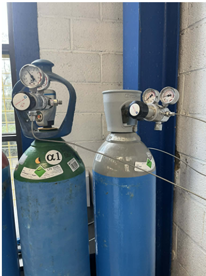
Figure 3.3: Argon and CO 2 cylinders supplying the CATLAB setup.
