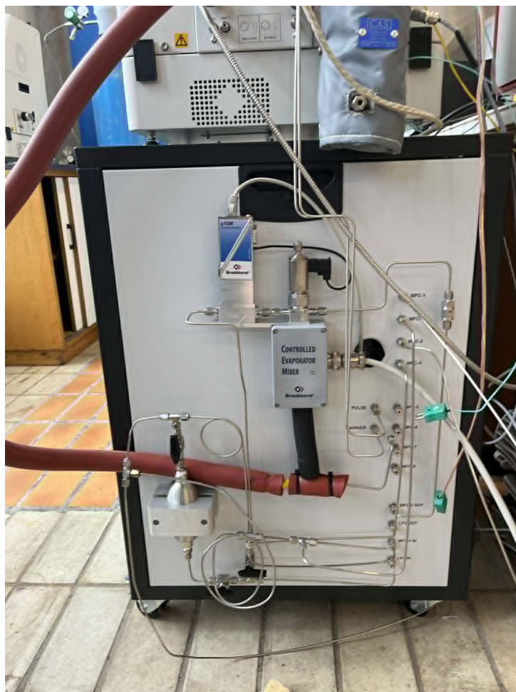
Figure 3.4: Gas distribution panel of the CATLAB system, showing the connections between the CATLAB and the gas line.
