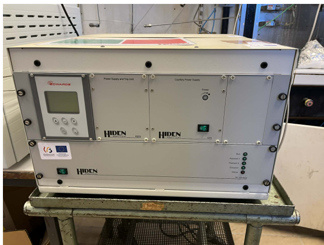
Figure 2.6: Hidden HPR-20 OEMS mass spectrometer used for online analysis of the micro-fixed bed reactor set-up effluent.
