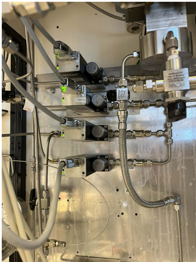
Figure 2.4: Mass flow controllers (Brooks Instrument) of the micro-fixed bed reactor set-up.
