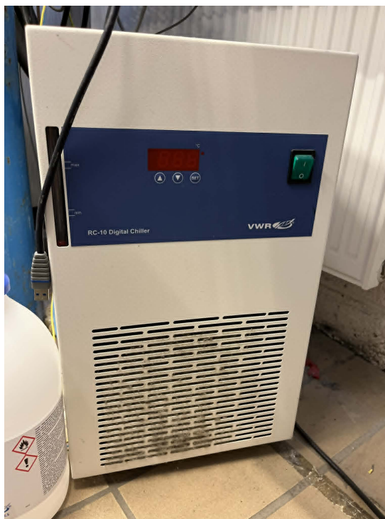
Figure 2.8: VWR RC-10 digital chiller used to condense water vapour at the micro-fixed bed reactor outlet.
