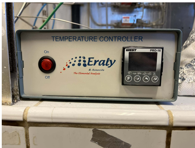
Figure 2.5: Early temperature controller used to regulate the micro-fixed bed reactor set-up furnace.
