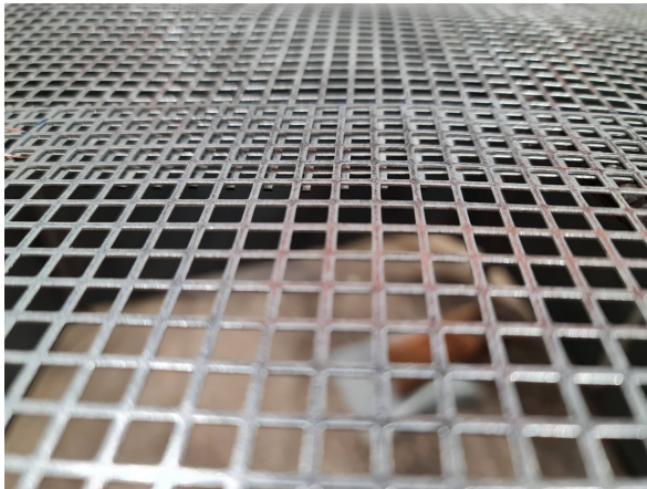
Figure 3.29: Mesh diffuser with 6 mm x 6 mm openings
