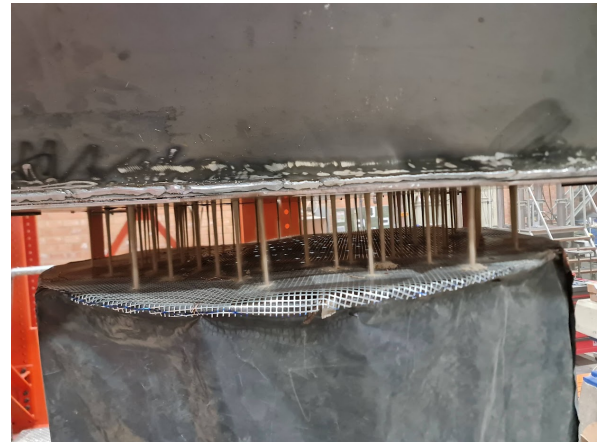
Figure 3.30: Pluviation process using the 6 mm mesh diffuser
