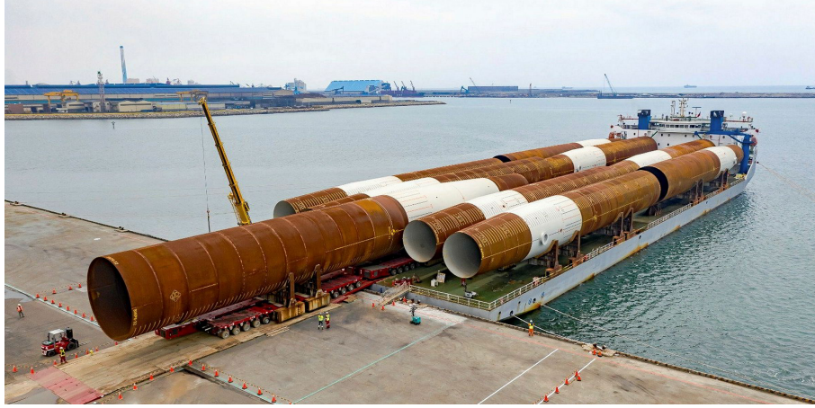
Figure 2.3: Monopiles in at Taiwan's first commercial offshore wind farm
