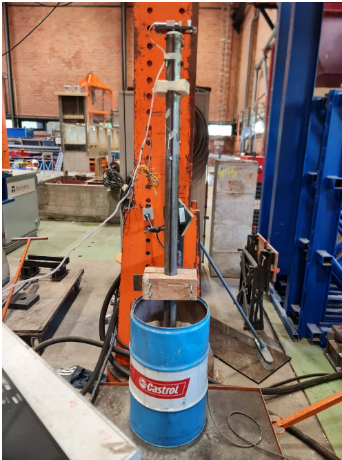
Figure 5.7: Vibro-driving test conducted in a 35 cm sand-filled reservoir, simulating offshore monopile installation.
