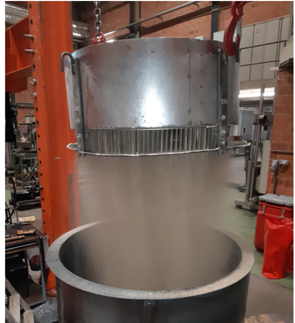
Figure 3.13: The old pluviometer system realised by Deckers Maxence and Defer Cédric [37].
