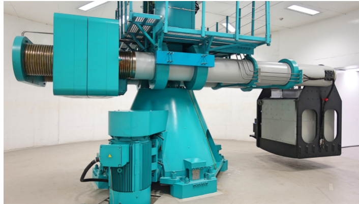
Figure 3.2: 5 m radius beam centrifuge at the University of Western Australia.
