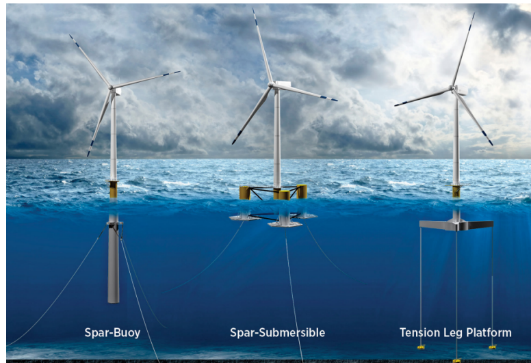
Figure 2.1: Types of floating offshore wind turbine platforms [27].
