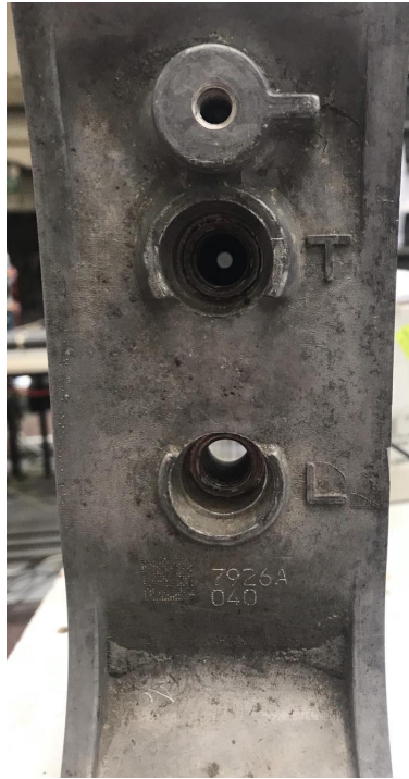
(a) Leading and Trailing spark opening
