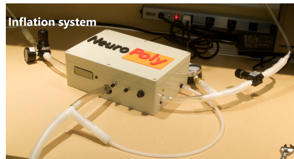
Figure 3.10: Pneumatic phantom for mimicking respiration-induced artifacts in spinal MRI developed by the Institute of Biomedical Engineering at Polytechnique Montreal [47]
