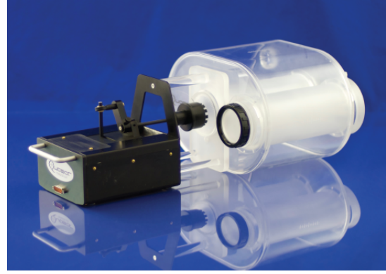
Figure 3.4: The programmable QUASAR™ MRI Motion Phantom [39]
