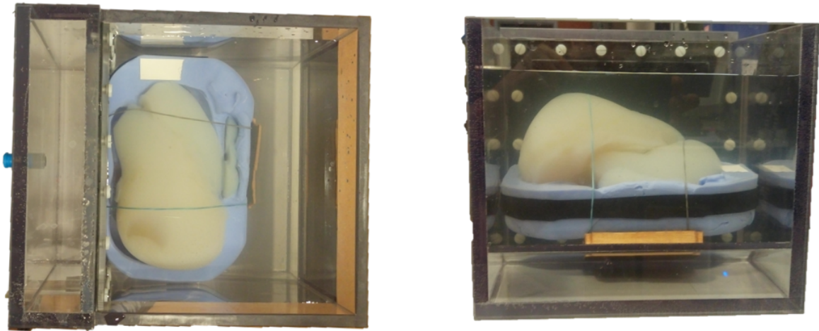
Figure 4.12: Liver with tumor, stomach and pancreas : Top view (left) and front view (right) of the phantom device
