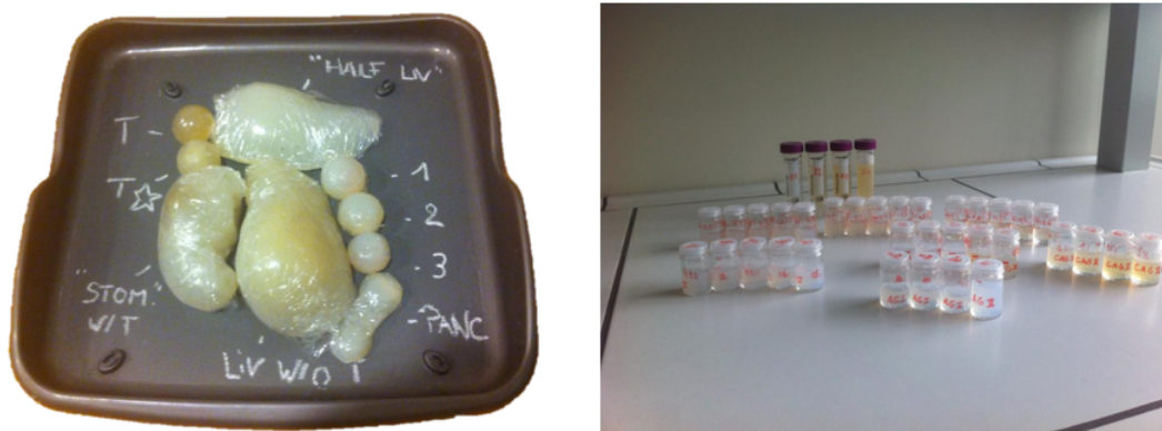
Figure 5.16: Organ-like gels prepared for an MRI scan (left) and test samples (right)
