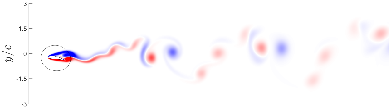
Fig. 4.12: Heaving airfoil - Re = 500 , A^* = 0.268 , F = 0.5 : dimensionless vorticity field \omega^* at t^* \simeq 51.76 , corresponding to t/T_f \simeq 7.75 . The plot is saturated for \omega^* > 6 . The limit between the FDoom and VPM results is represented by a thin black line.
