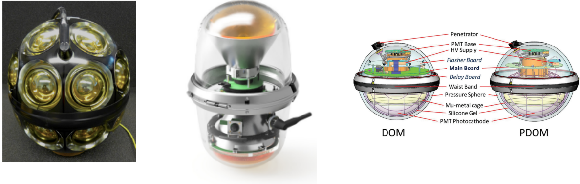
Figure 3.2: Illustrations of the mDOMs (Abbasi et al., 2021), DEggs (Abbasi et al., 2023a), and PDOMs (Nagai and Ishihara, 2019) used for the IceCube Upgrade.
