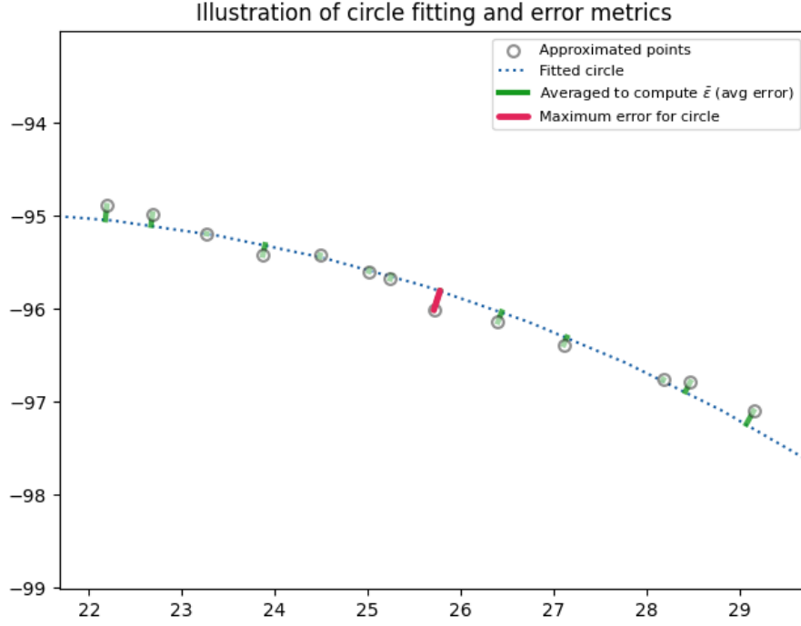
Figure 1.9: Illustration of circle fitting and error metrics on a single arc of a violin outline. Each green segment is the individual error |||p_i - \mathbf{c}_k|| - r_k| for one contour point p_i . The magenta segment highlights the maximum error on this arc. Note that the evaluation metrics are computed over the full outline; this view shows a single arc for clarity.
