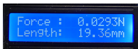
Figure 4.19: Display of the force and position on the 2x16 LCD screen.
