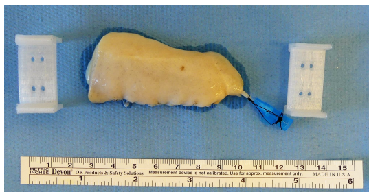
Figure 4.29: Graft and both removable graft attachment pieces.
