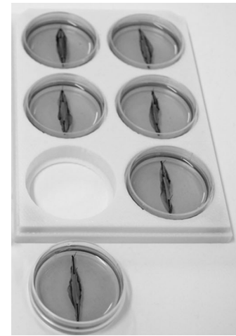
Figure 1.8: Donnelly's 3D muscle-stimulating bioreactor. Used tissues: C2C12 cells in fibrin between two silk sutures [29].
