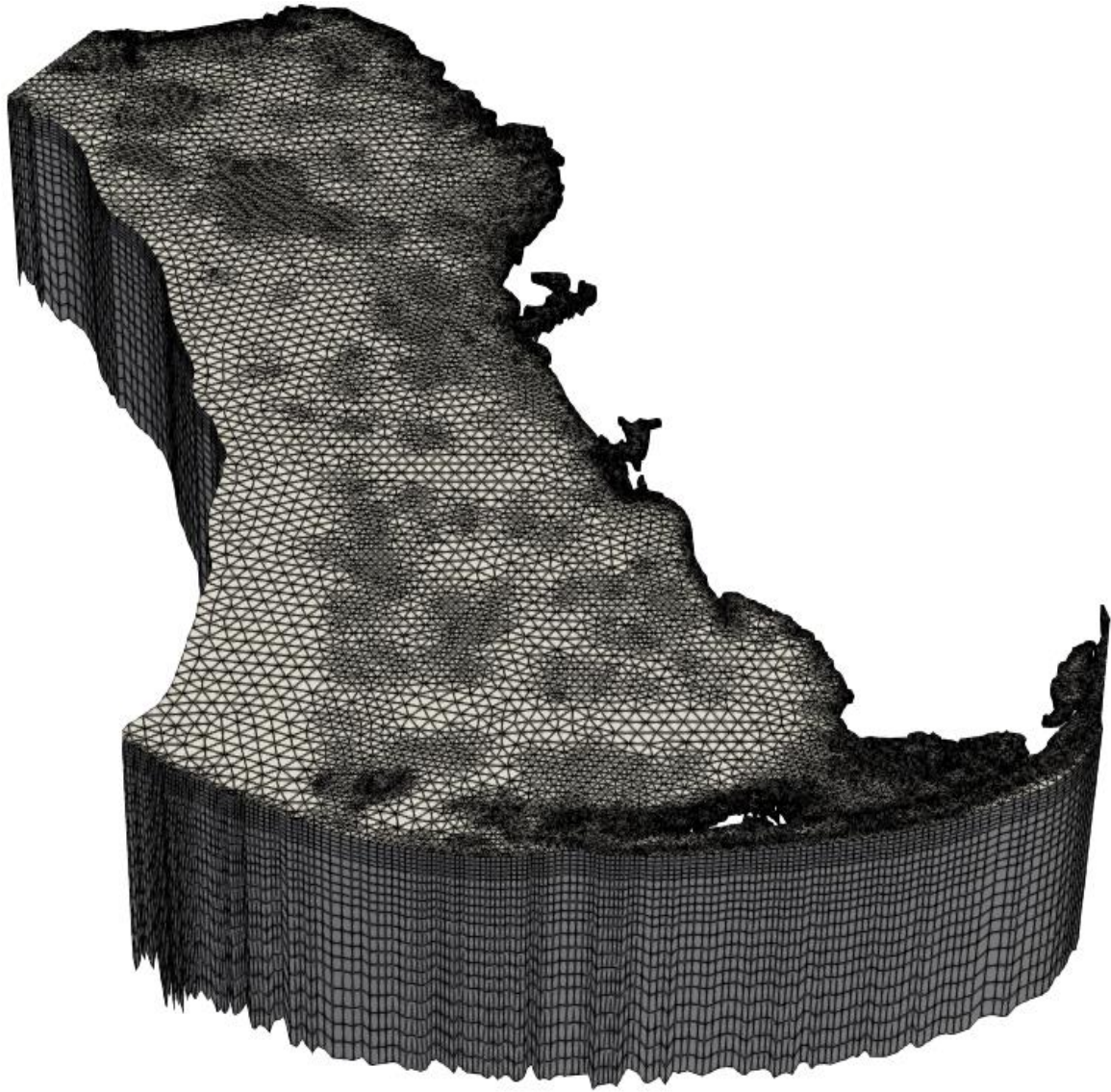
Figure 6 : 3D-mesh of the computational domain There are 20 \sigma levels. The dark black lines represent the limits between elements.
