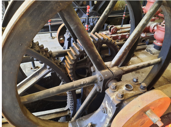
Figure D.4: Driven gear of the reduction of 1:4
