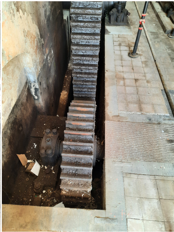
Figure D.2: Driven gear of the reduction of 1:5
