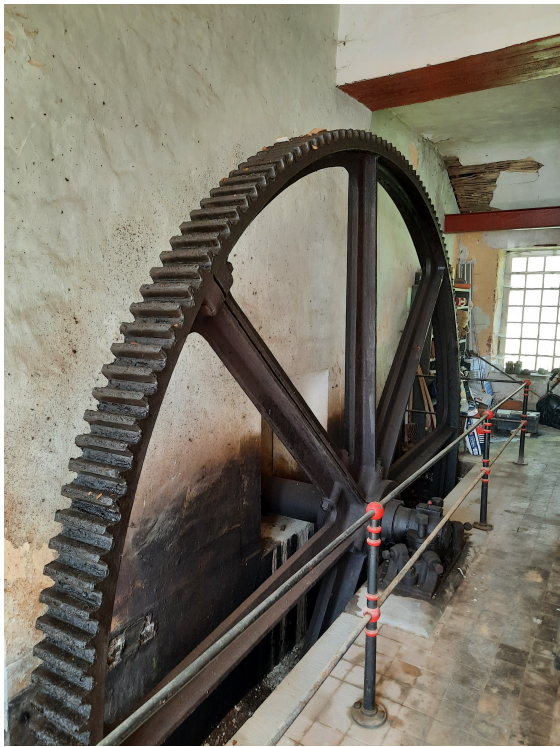
Figure D.1: Drive gear of the reduction of 1:5
