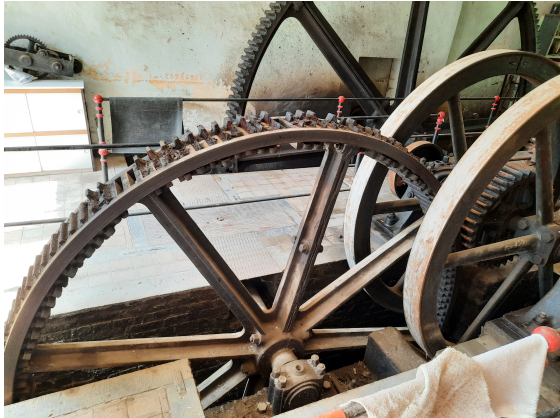
Figure D.3: Drive gear of the reduction of 1:4 (fail wheel)
