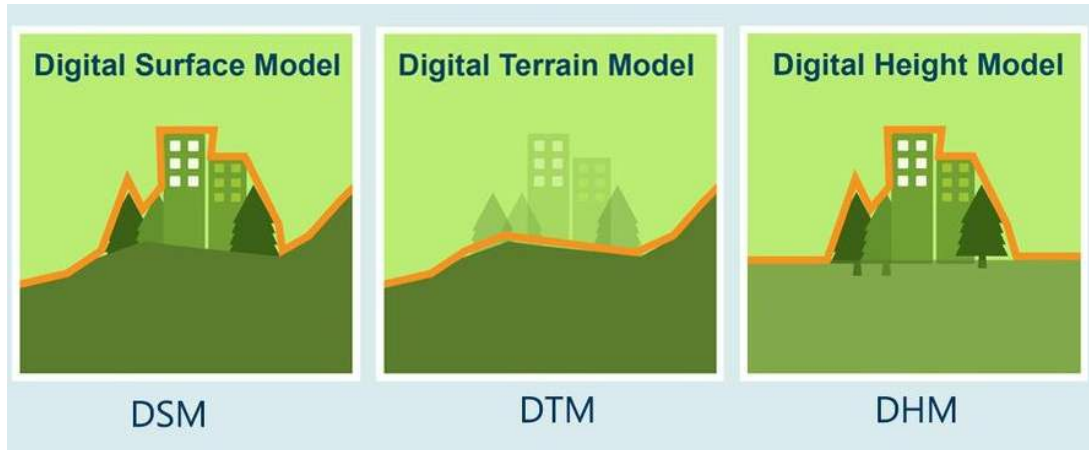
Figure 4.2: Schematic representation of the derivation of the DHM from the DSM and DTM (source: GeoSun Tech (n.d.))
