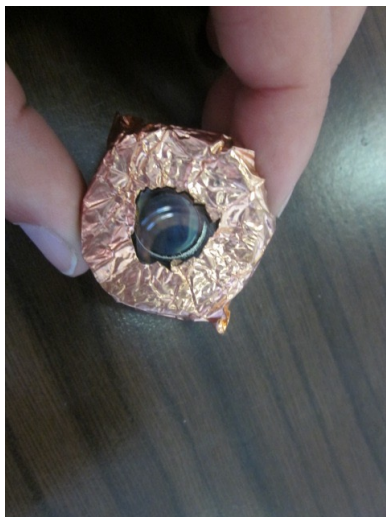
FIGURE 3.1: Electrical contact made by a copper sheet in front of the sample.
