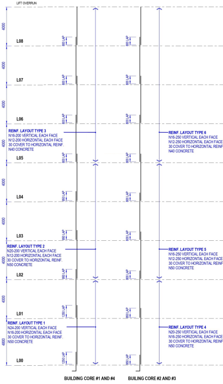
Figure 4.8: Layout of vertical reinforcement for the four cores, adapted from the given plan.
