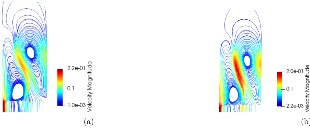
Figure 4.15: streamlines just above the channels of the uniform heating profile (b) and the sinusoidal heating profile (a) at t = 110s
