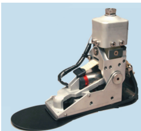
Figure 1.8: Power ankle-foot prosthesis with SPEA [21]
