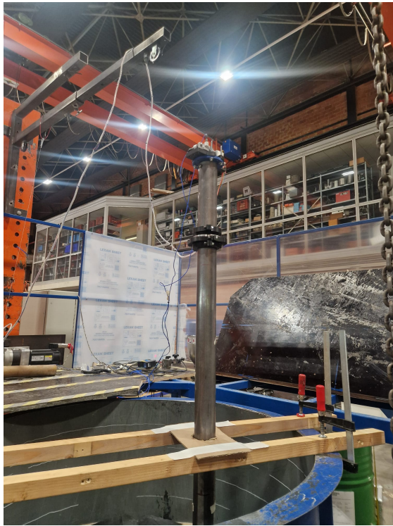
(a) General view of the vibratory driving arrangement.
