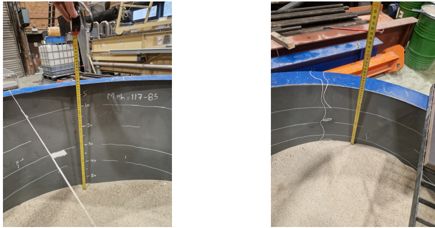
Figure 21: Examples of height measurements in the large tank after pluviation and before levelling.
