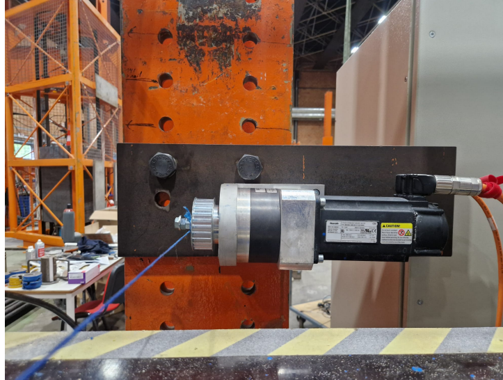
Figure 46: Motor-driven system used to impose the lateral displacement during the loading tests. The Bosch Rexroth servo motor is coupled to a planetary gearbox and drives the winding drum connected to the Dyneema cable.
