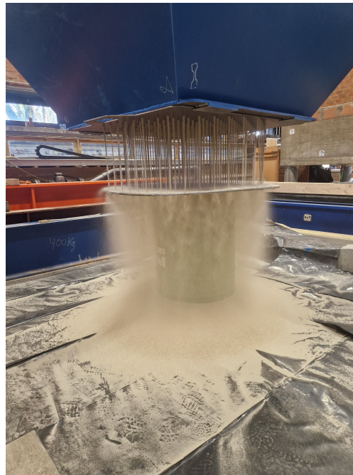
Figure 24: Pluviation in progress.
