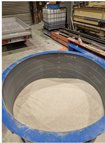
Figure 20: Surface of the sand mass in the large tank immediately after pluviation.
