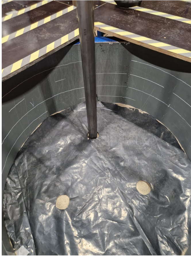
Figure 57: Tarpaulin used to materialise the three pile locations at the surface of the sand mass.
