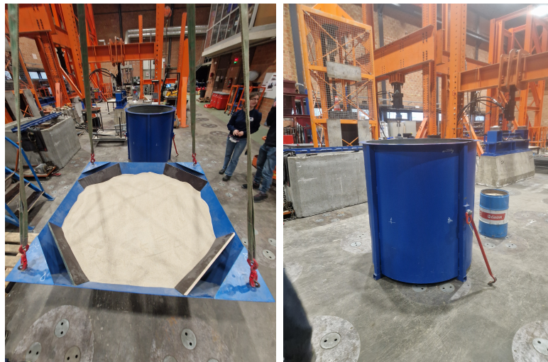
Figure 17: General view of the large tank used for the pluviation test and of the existing pluviation system available in the laboratory.
