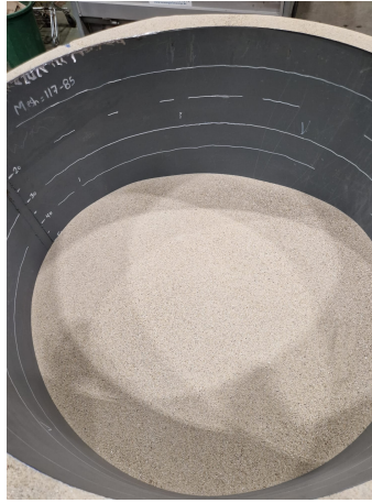
Figure 34: Surface of the sand mass in the large tank immediately after pluviation.
