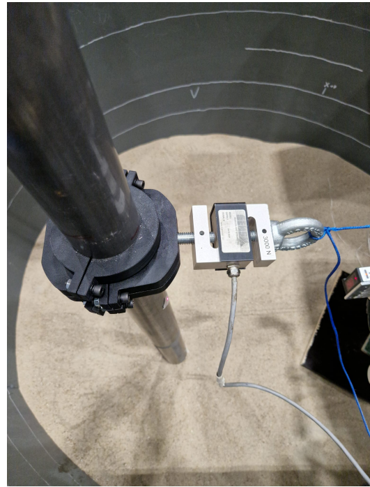
(b) Detailed view of the force sensor connected to the load-transfer device.
