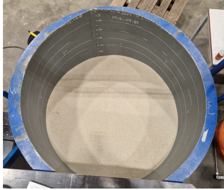
Figure 36: Surface of the sand mass in the large tank immediately after pluviation.
