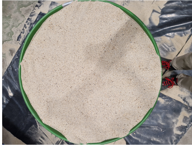
Figure 28: Top view of the final sand surface after the second pluviation test in the small tank.
