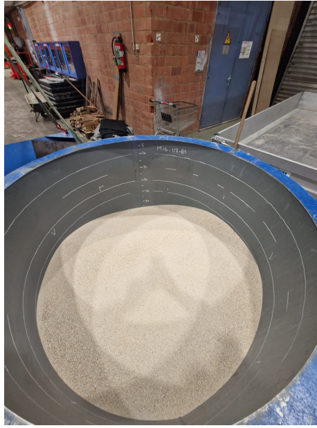
Figure 31: Surface of the sand mass in the large tank immediately after pluviation.
