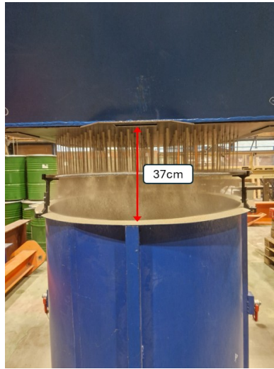
Figure 18: Measured free-fall height in the large-tank pluviation setup.
