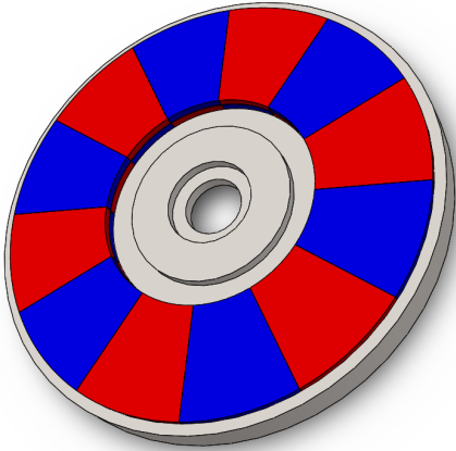
Fig. 3.4: SOLIDWORKS view of the rotor with the PMs arrangements.
