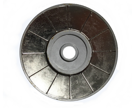
Fig. 3.5: Picture of the rotor with the PMs arrangements.
