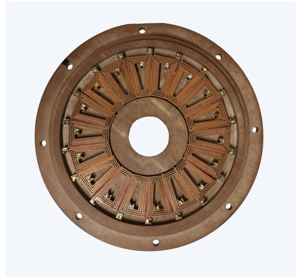
Fig. 3.9: Picture of the 18 coils constituting the stator windings.
