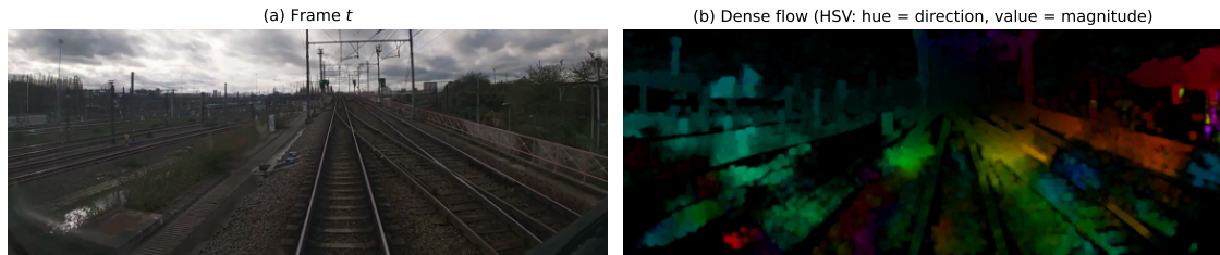
Figure 2.7: Dense Farneback optical flow on a railway frame. (a) Source frame at time t . (b) Flow field in HSV: hue encodes the direction of the per-pixel displacement, brightness its magnitude.
