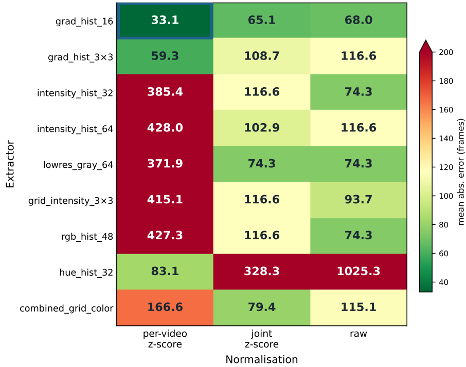
Figure 5.6: Mean absolute alignment error (in frames) on the Plan 2 ground truth across the cartesian product of nine extractors (rows) and three normalisation regimes (columns). The best cell — grad_hist_16 with per-video z-score, 33.1 frames — is highlighted; gradient-histogram extractors with per-video normalisation dominate the low-error region.
