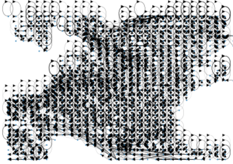
Figure 2.4: Lagrangian flow network of low resolution 30x30 subdomains, 120 particles in each box
