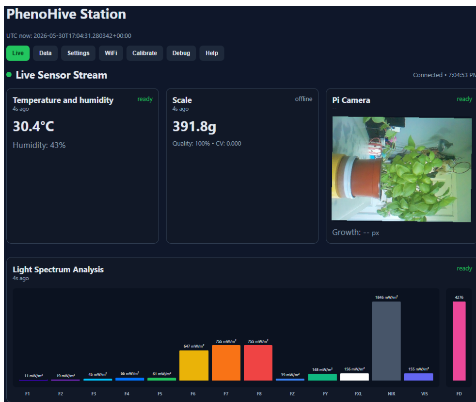
Figure 8.2: The Debug UI live tab showing real-time readings from all sensors. The spectral bar chart (bottom) visualizes the live data from the 14 TCS3448 channels. The temperature, humidity and weight live values are displayed as large numeric cards. The interface refreshes every few seconds via Asynchronous JavaScript and XML (AJAX) polling.
