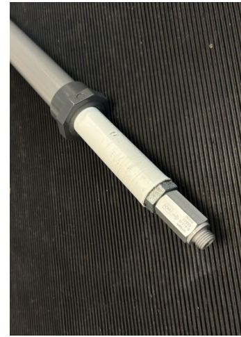
(c) Installed one-way valves for airflow regulation at both ends.
