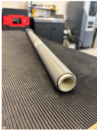
(a) Piston tube assembly showing the piston inserted into the vacuum chamber.
