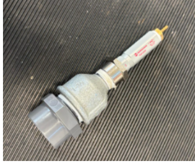
Figure 4.4: Stepwise reduction from the main body to the 6mm tubing connection using reducer fittings and a one way check valve.
