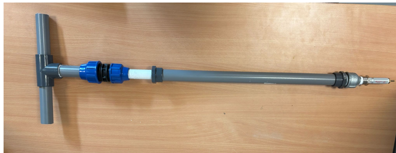
Figure 4.5: Fully assembled PVC suction pump.
