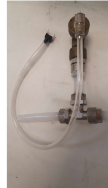
(d) Tubing and connectors with a pressure transducer (in black).
