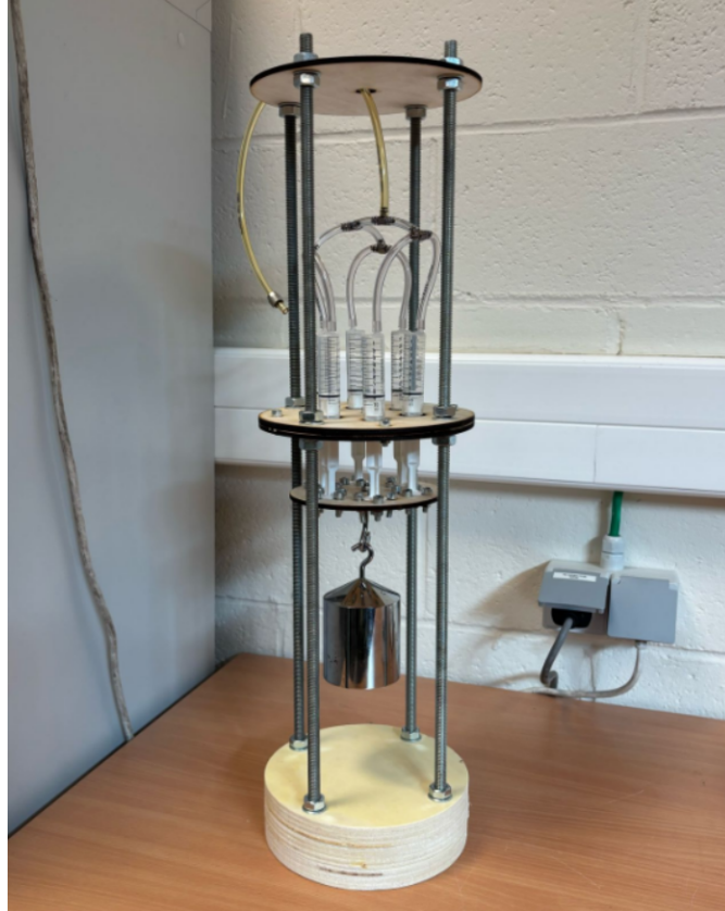
Figure 4.9: Fully assembled syringe-based vacuum pump.
