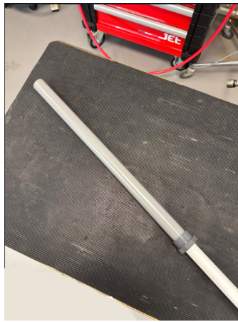
(b) Main body assembly with 1-inch adapter sealed at the handle end.
