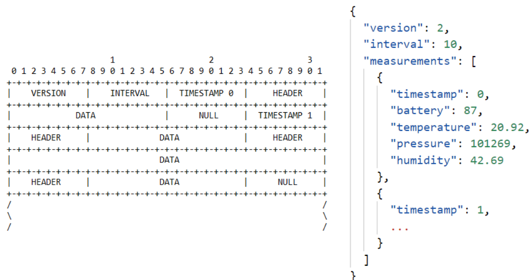
Figure 3.8: Packet format V2. Left: LoRaWAN payload; right: JSON object
