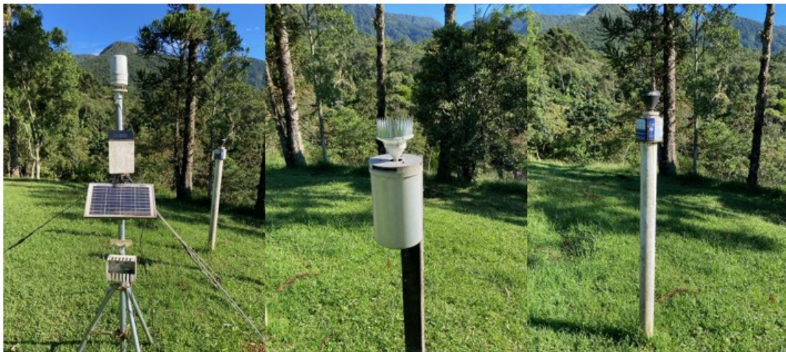
Figure 9: HOBO weather station (INPE) at the São Francisco Xavier study site. (a) Main tripod with cup anemometer, radiation-shielded T/RH probe, solar panel and datalogger (+ barometric sensor). (b) Tipping-bucket rain gauge. (c) Pyranometer. Taken by Lucas Jeangout, 13/02/2026.
