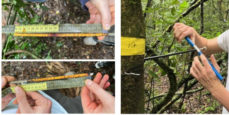
Figure 13: Extraction of wood cores with an increment borer (right). Left up, visible colour differentiation between heartwood and sapwood, Left down, no colour differentiation visible.
