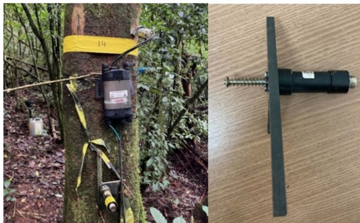
Figure 10: Left: sap flow (up) and dendrometer (down) sensors positioned on tree 14, Right: dendrometer sensor.
