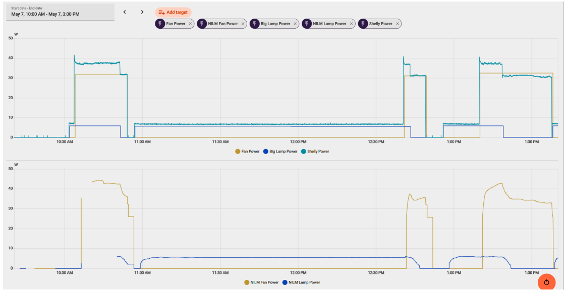
Figure 4.1: End-to-end qualitative validation in Home Assistant. Top : ground-truth power recordings from the smart plugs on the fan (yellow) and lamp (blue), and the household aggregate signal from the Shelly Pro EM (cyan). Bottom : per-appliance disaggregation estimates produced by the deployed NILM service and ingested as Home Assistant sensors.
