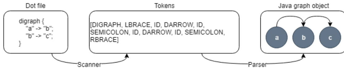
Figure 4.4: Illustration of the dot parsing process
