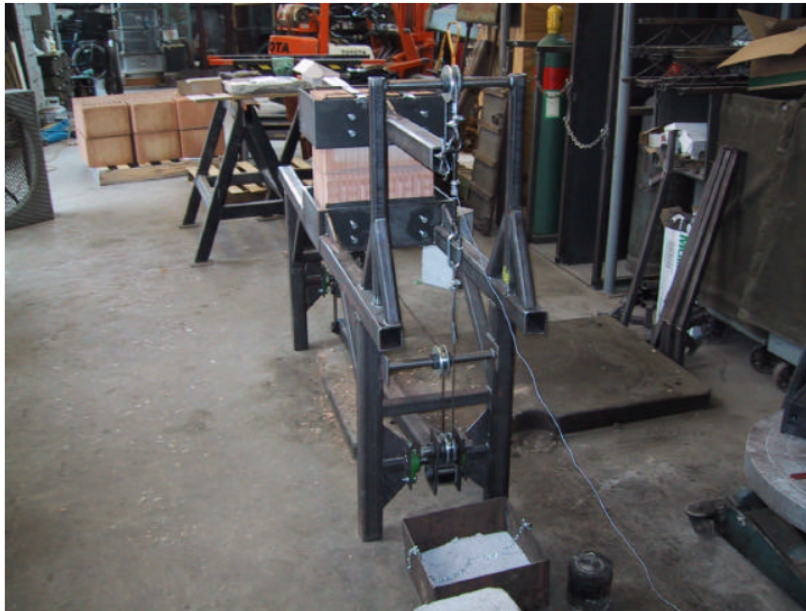
Figure 4.14: Pure couple bond wrench apparatus: General view [49].
