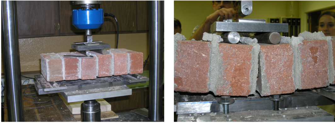
Figure 2.1: Beam test execution [3].
