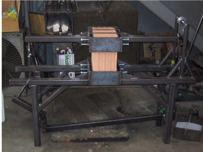
Figure 4.12: Pure couple bond wrench apparatus: Side view [49].
