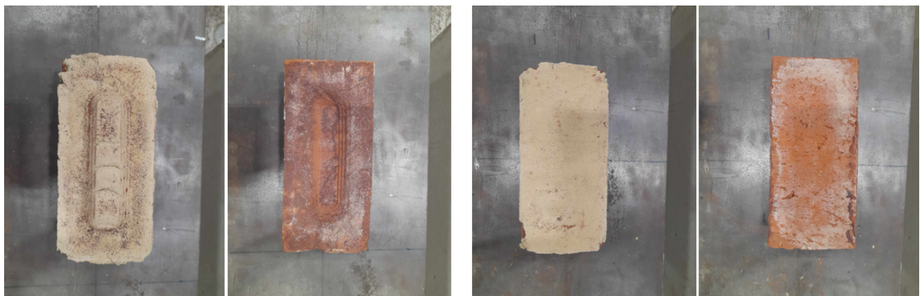
Figure 4.7: Failure modes observed during the study. Mode 1 on the left, mode 2 on the right.
