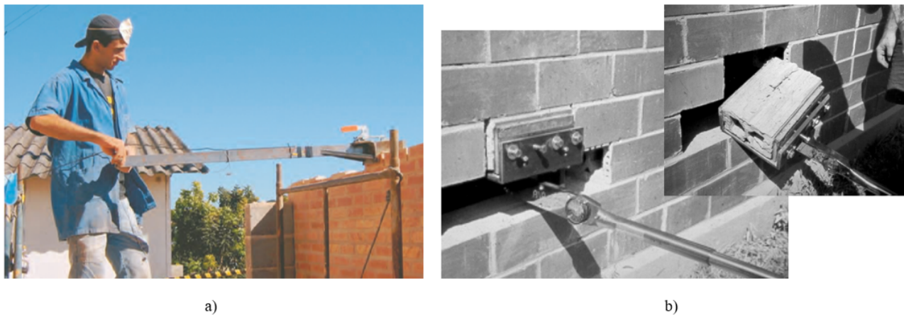
Figure 2.20: In-situ bond wrench testing [50, 51].
