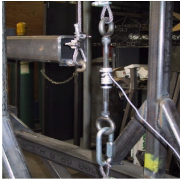
Figure 4.16: Pure couple bond wrench apparatus: Load cell [49].
