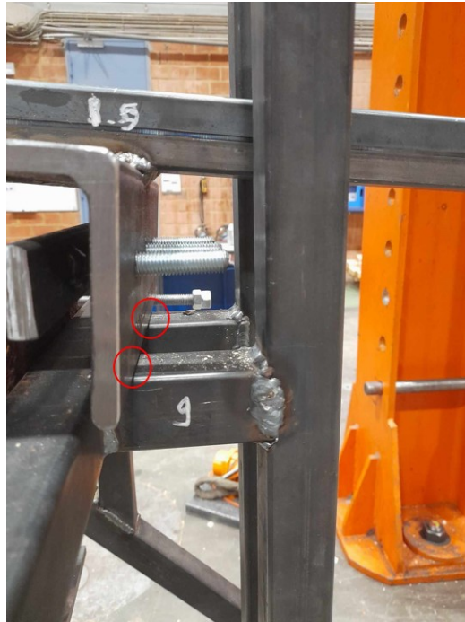
Figure 3.15: Lever arm in contact with the apparatus frame during testing.
