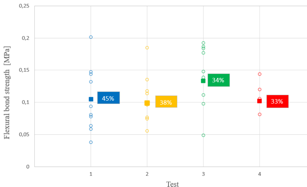
Figure 4.1: Flexural bond strength by test type.
