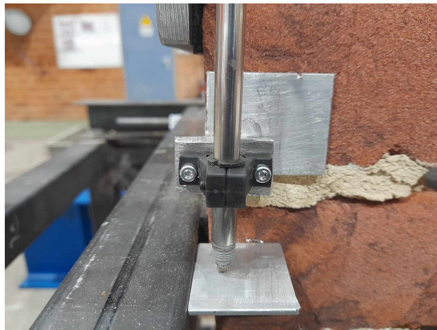
Figure 3.12: Placement of LVDT, targeting the area of maximum tensile strain.
