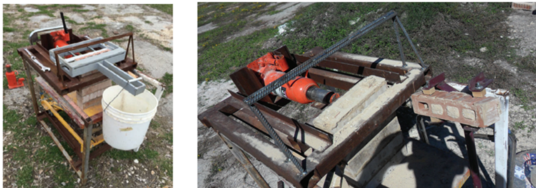
Figure 2.13: On the left: the ASTM C1072 apparatus loaded with a bucket. On the right: The AS 3700 apparatus after the failure of a joint. [6]
