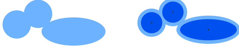
Figure 3.4: On the left, a binary image that consists of one connected component. On the right, the different objects in that image, distinguishable due to the concavities in the foreground's edges.
