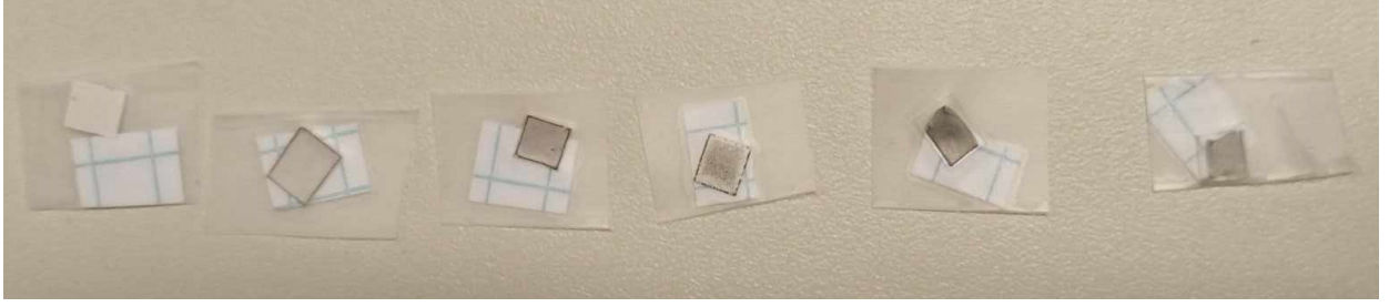
Figure 4.13 – MNP samples. The sample in the foreground, and its labeling on a simple grid in the background. Total thickness with foil and tape \approx 1 mm.
