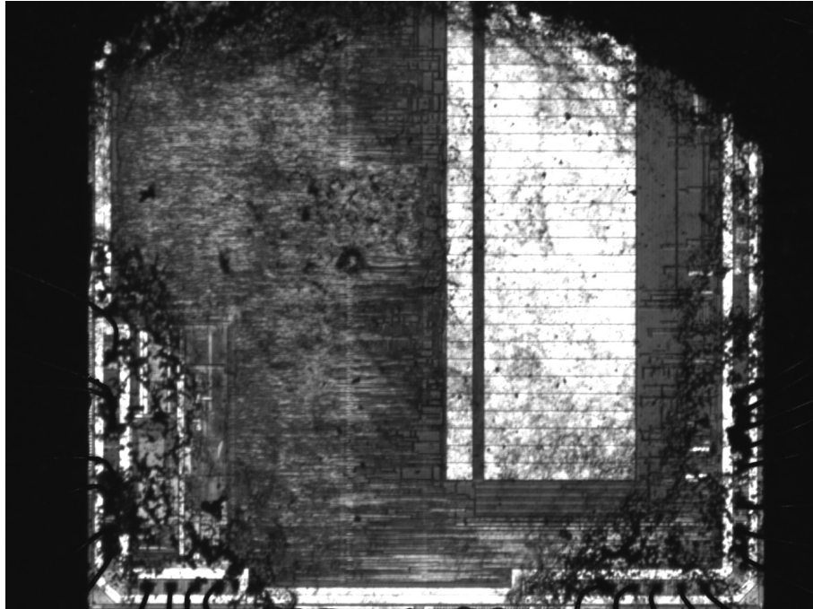
FIGURE 5.2: Microscope view of a depackaged AT644P
