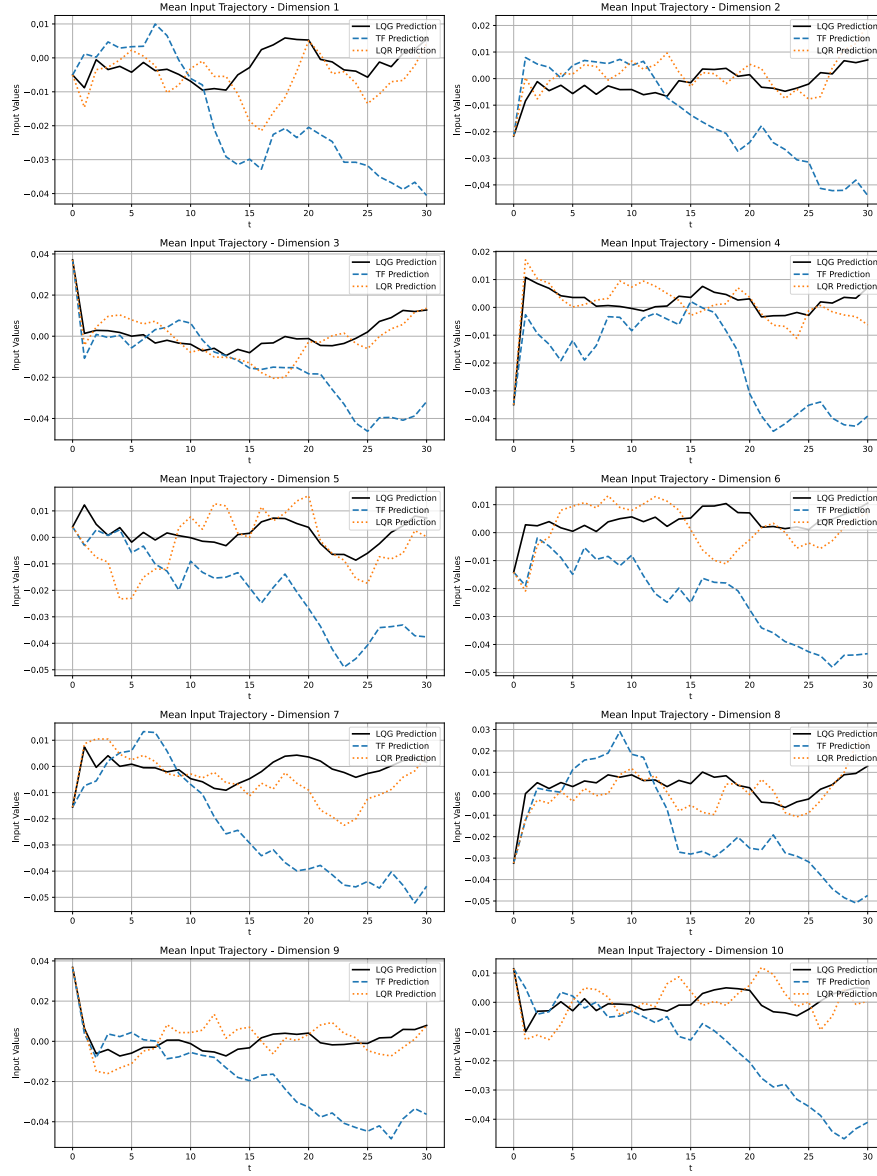
Figure 5.10: Trajectories of internal state components over the trajectory horizon and shown separately for the n_x state dimensions for each method except the the naive proportional controller: the optimal LQG controller, the Transformer-base model (TF) and LQR, and for LTI systems with non-i.i.d. Gaussian noise.
