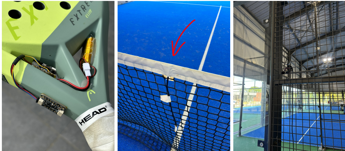
Figure 3.3: ( left ) IMU subsystem placement ( center ) contact microphone sensor placement ( right ) airborne microphone placement
