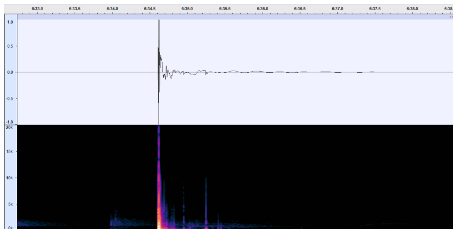
Figure 5.4: Example contact microphone waveform and spectrogram from the annotation test
