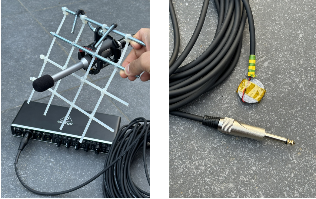
Figure 5.1: ( left ) ECM8000 microphone with the custom mount and audio interface ( right ) Contact microphone
