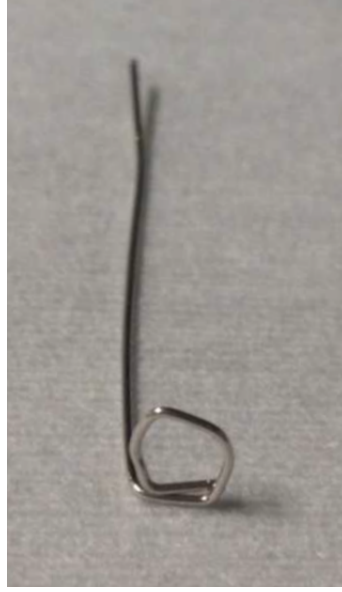
Figure 4.4: Shape of platinum counter-electrode used for electrochemical etching. The circle is around 2.3 mm.
