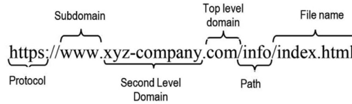
Figure 2.5: Structure and components of a URL from Sahingoz et al. [17].
