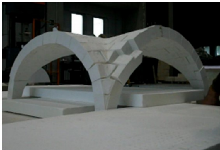
Figure 2.8: Limit state before collapse: damage mechanism [8]
