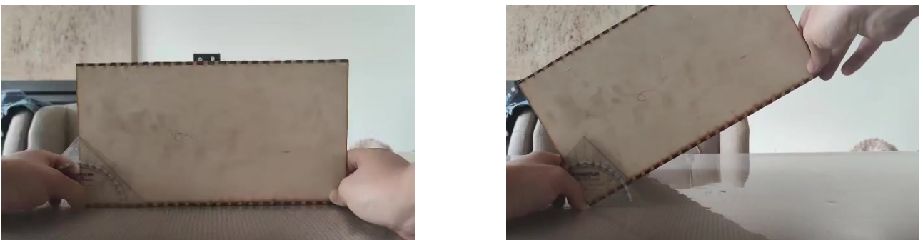
Figure 5.1: Friction coefficient measurement at start and finish
