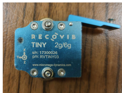
Figure 3.21: Accelerometer Recovib Tiny
