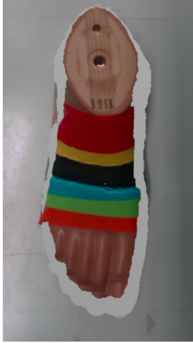
Figure 3.14: To simulate the tattoo, colored sheets of paper are fixed on a foot prosthesis
