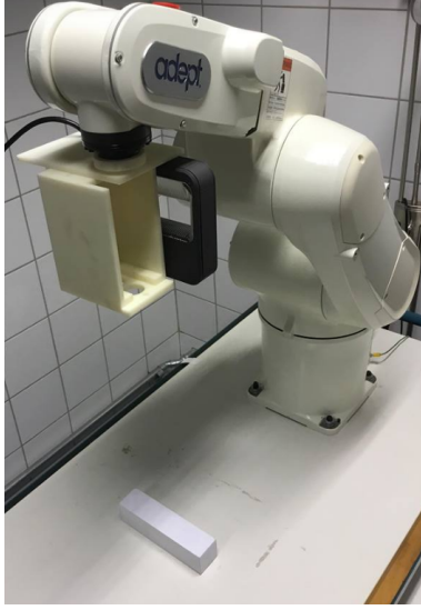
Figure 3.29: Scan of a reference object with known dimensions
