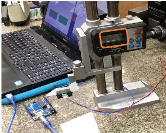
Figure 2.37: SHARP fixed to a measuring column
