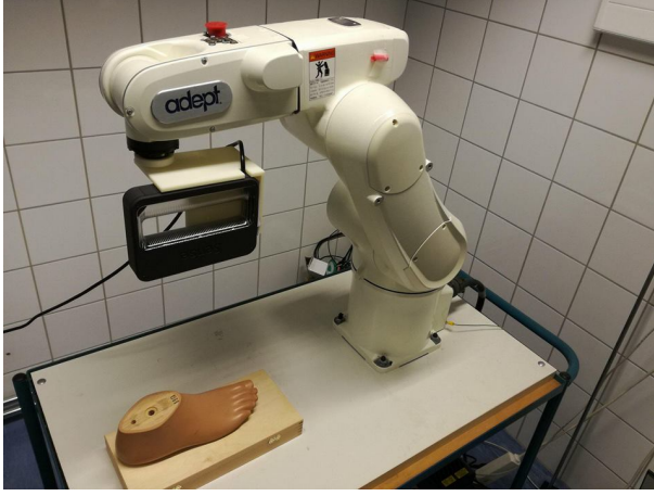
Figure 2.12: Robot scanning a foot prosthesis without moving at 35cm
