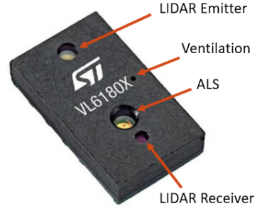
Figure 1.43: VL6180X sensor using ToF [38]
