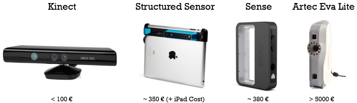
Figure 1.20: Products using structured light technology available on the market [34]
