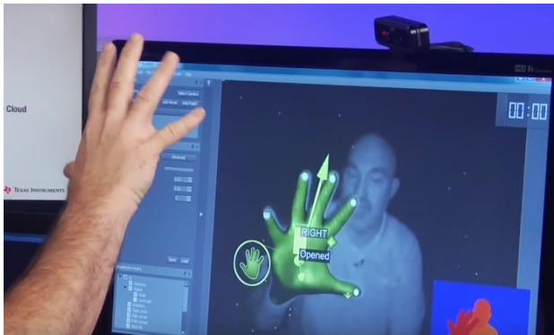
Figure 1.15: Test of the TEXAS INSTRUMENTS™ ToF camera [25]
