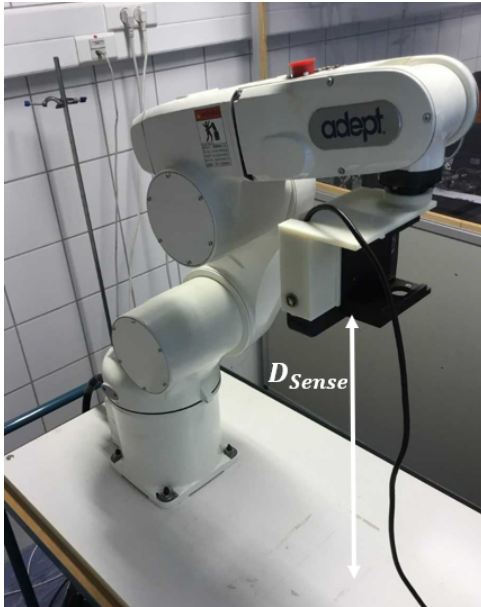
Figure 2.10: Position of the robot where the end-effector is above the table and D_{Sense} is limited to 50 cm
