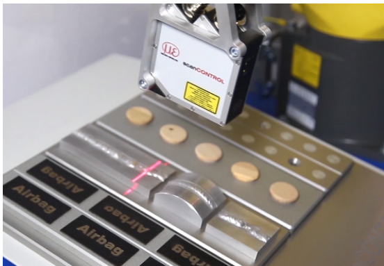
Figure 1.4: Laser triangulation scanner of MICRO-EPSILON ® fixed on a robot scanning a welding [8]
