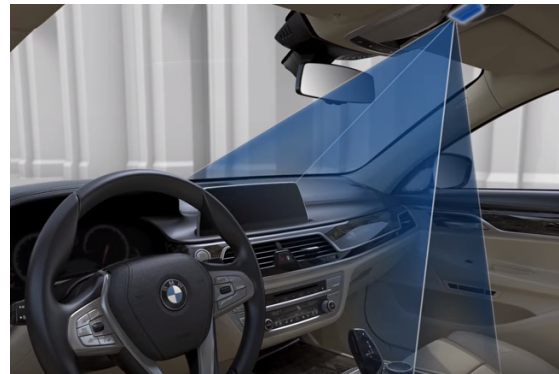
Figure 1.16: System of gesture control of BMW® using ToF [23]
