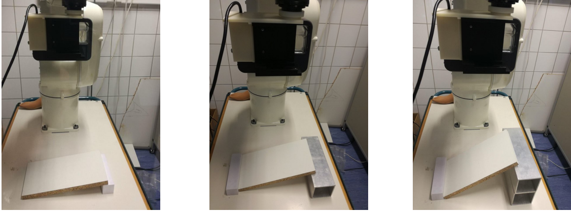
Figure 3.22: Experiment where the SENSE scans a plate with three different angles : 8.3^\circ , 16.5^\circ and 34.6^\circ
