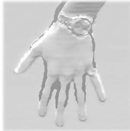
Figure 3.8: Influence of reflecting objects like a metallic watch and a metallic ring
