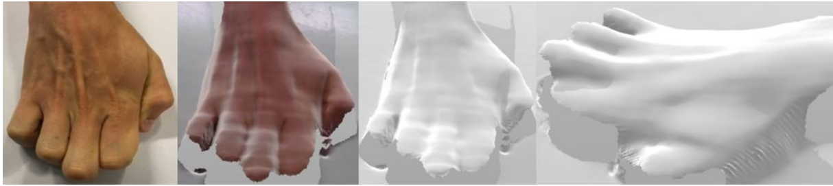
Figure 2.17: Scan at 50 cm with a movement of rotation and translation trying to detect skin irregularities
