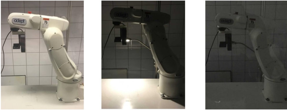
Figure 3.1: Experimental setup for testing the SENSE in different lighting conditions : classical lighting (neon lights), spot and no lighting
