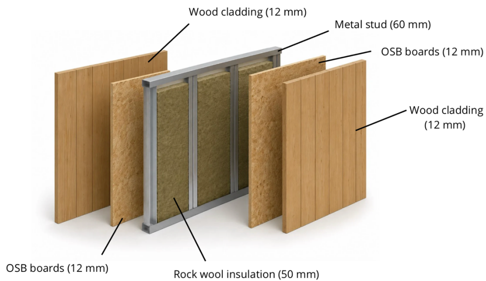
Figure 17: Layered composition of a hybrid wall with wood finish
