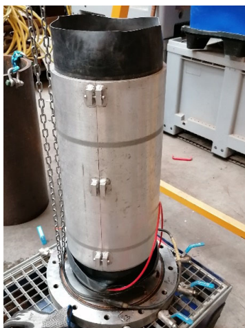
Photo 5 – 6 – 7: Sample placement on the load cell and removal of the mould
