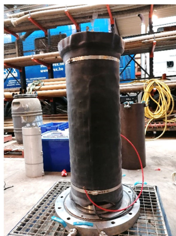
Photo 5 – 6 – 7: Sample placement on the load cell and removal of the mould
