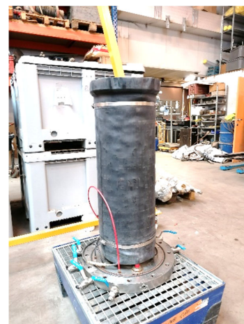
Photo 5 – 6 – 7: Sample placement on the load cell and removal of the mould
