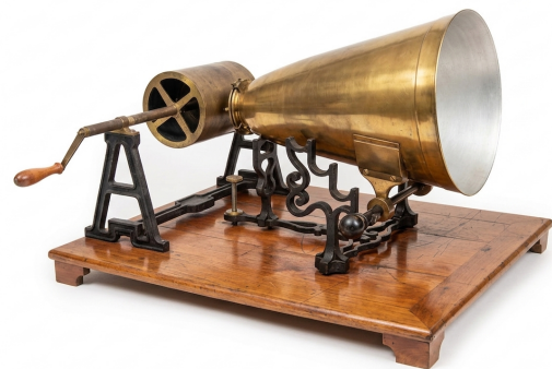
FIGURE 2.1 – Le Phonautographe de Léon Scott de Martinville (1857) [1]
