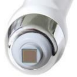
Figure 1.5: The Corneometer is the worldwide most used probe to measure skin hydration.[11]
