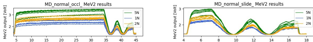
(a) Evolution of MeV2 output in the "occlusion" condition. It is characterized by an increase during the occlusion time on the right patch followed by two other peaks corresponding to the middle and left patches (b) Evolution of MeV2 output in the "slide" condition. It is characterized by three peaks corresponding to the different patches, going from right to left.
