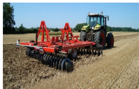
Figure 1.3: Disc ploughing. Adapted from QUIVOGNE (n.d.), https://tinyurl.com/nhhev2sy .
