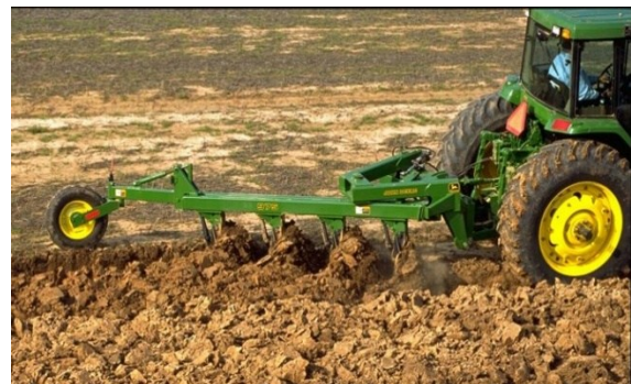
Figure 1.5: Moldboard ploughing. Adapted from Riechmann Bros (n.d.), https://tinyurl.com/4zfnty49 .
