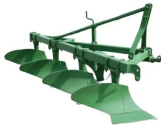
Figure 1.4: Moldboard plough. Adapted from JCBL (2024), https://tinyurl.com/bdd6yjf5 .
