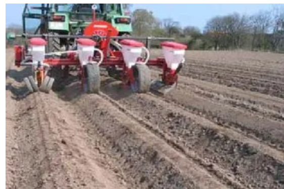
Figure 1.7: Ridge tillage, Adapted from Kristensen et al., 2006.
