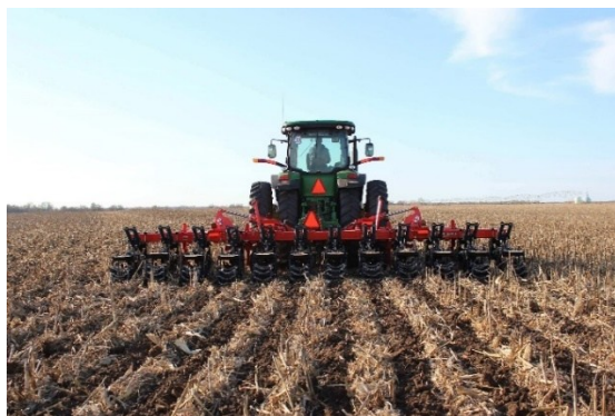
Figure 1.6: Strip till, Adapted from KUHN (n.d.), https://tinyurl.com/nhhwakza .
