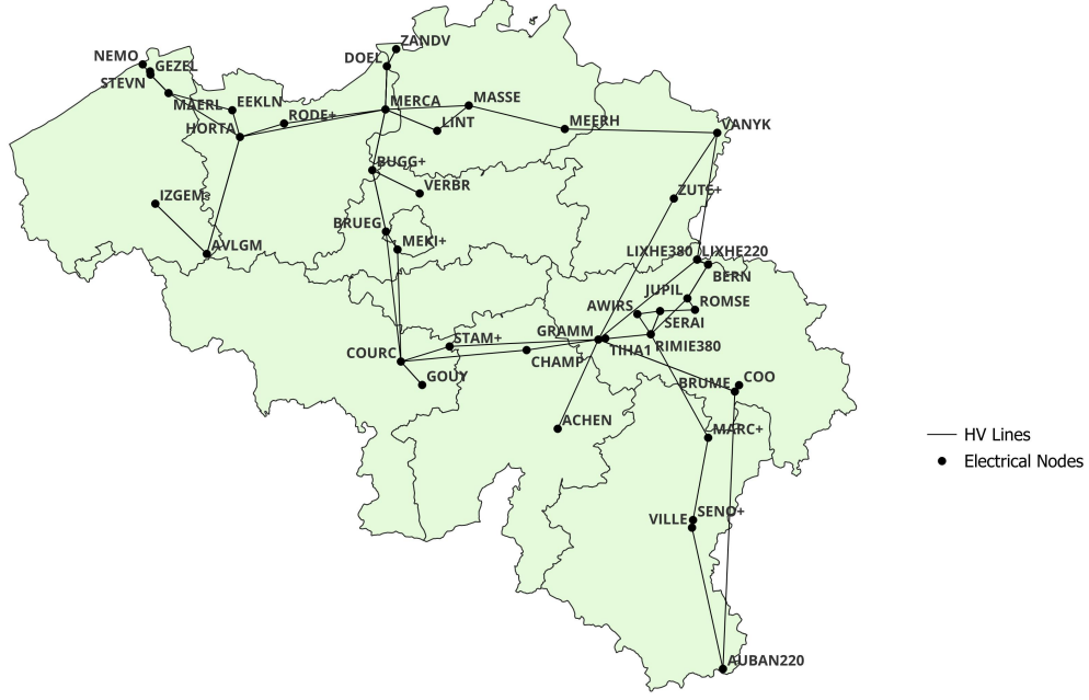
Figure 4.1: Implemented Electrical Grid
