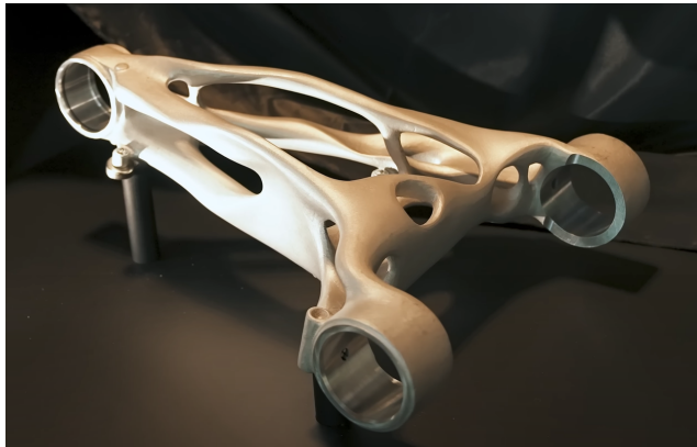
(a) Bugatti Tourbillon suspension wishbone, figure from [9].
