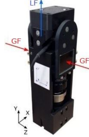
Figure 8: Decomposition of the force applied by the fingers on the manipulandum into grip force (GF) and load force (LF). [3]
