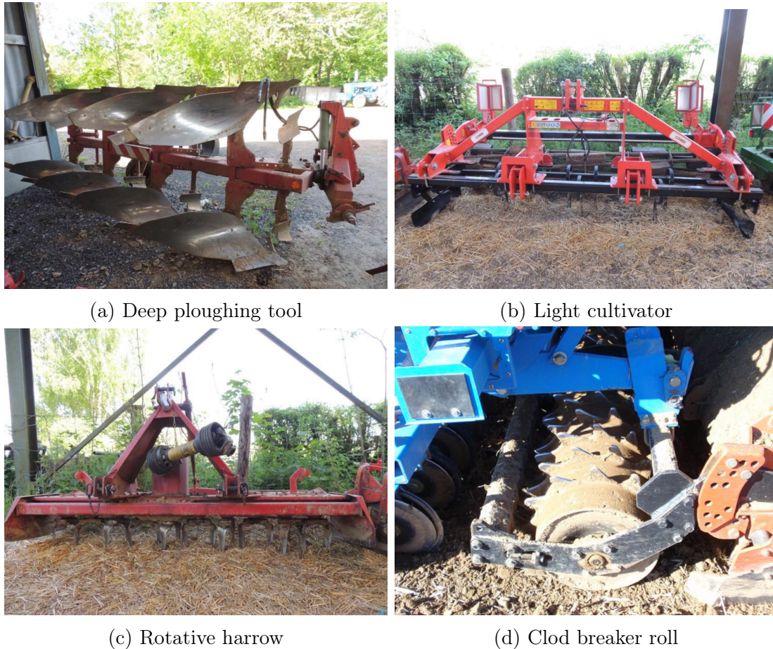
Figure 1.2: Different tools commonly used in conventional farming soil management practices (Bertin, 2023)
