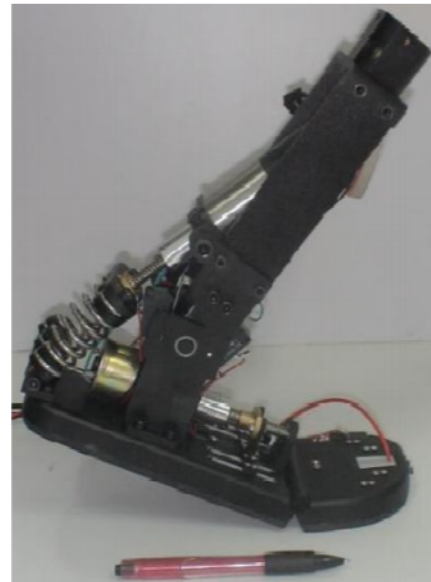
Figure 2.14: The CAD models of PANTOE 1 with compliant joints and a segmented foot (left) and the prototype of PANTOE 1. It is made of aluminum-alloy [27]
