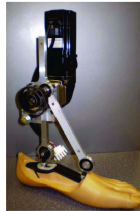
Figure 2.12: Four bar foot prosthesis prototype [26]
