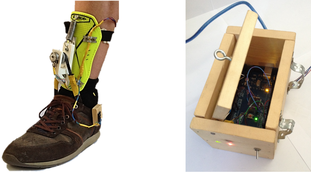
Figure 3.5: Mechanical part (left) and electronic part (right) of the optimal mechanism
