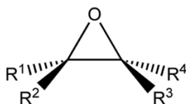
Figure 4 - General structure of a substituted epoxide (oxirane).
